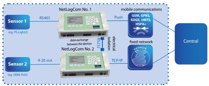
The input channels (W, W1) can be monitored continuously via differential channels in the **NetLogCom**. If the channels drift apart for instance or in the event of an error message (faulty sensor) an instantaneous alarm signal is sent according to the previously established alarm configuration. This signal can be sent by: SMS, FAX, voice prompts, e-mail). Data can be retrieved via the HTTP server, even if it is password protected.
