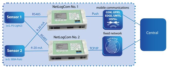
4) 2 Logger, 2 transmission paths, 2 sensors (hydrological, meteorological or agro-meteorological sensors), (with serial data verification)
